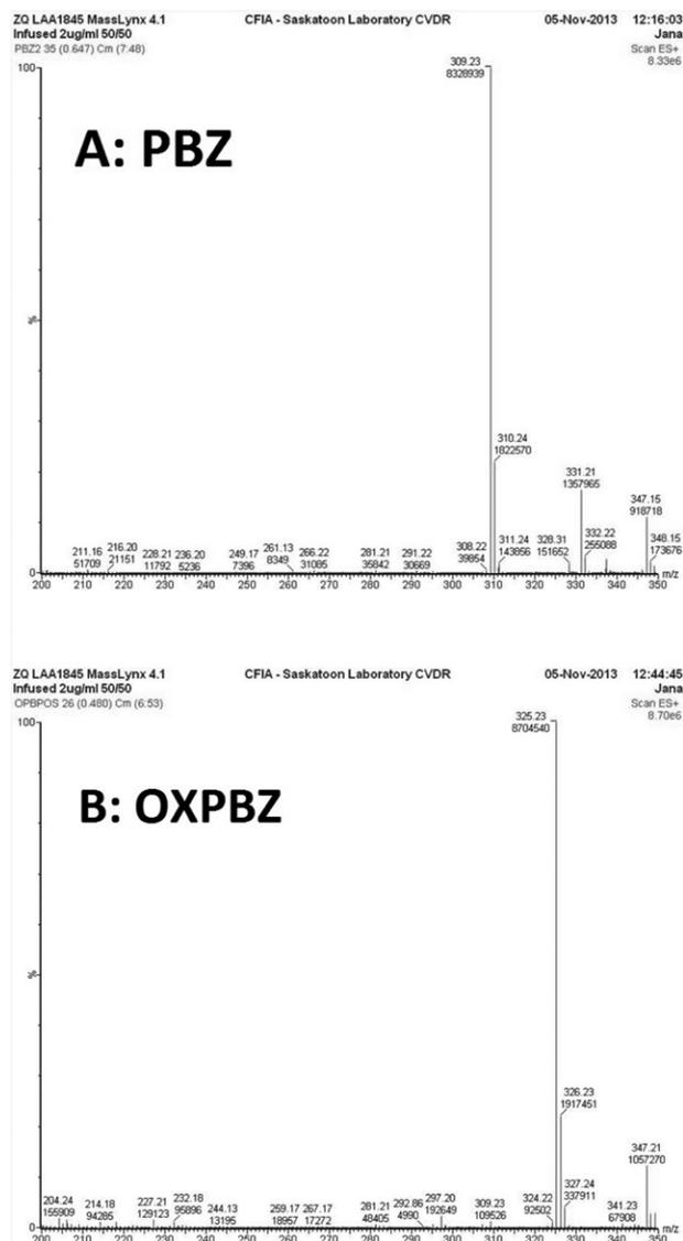
Figure 2. Mass spectra of PBZ and OXPBZ.
